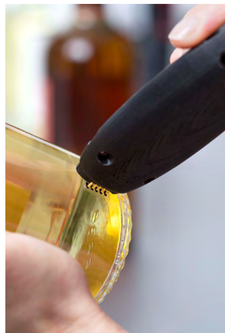
An example of Xerox printed memory being read with a device.
