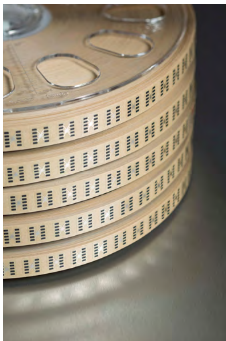
Xerox printed memory in web format (left) and in single track rolls (right).
