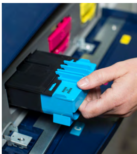
An example of Xerox printed memory on a printer cartridge.
